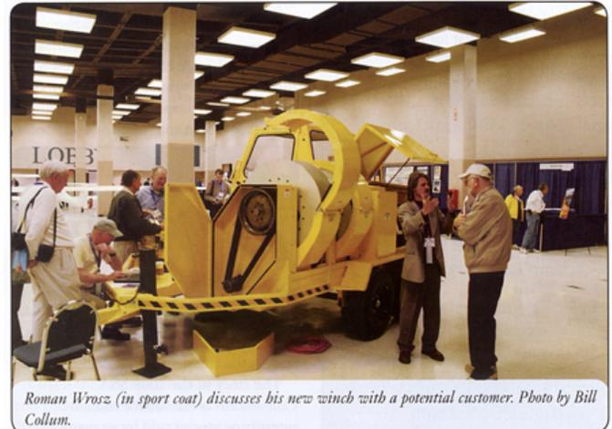
As Roman was giving me a tour of the 2drum model on display, I couldn't help but notice that the thing looked like it was armored, with heavy steel doors and covers. It even uses a blank rifle cartridge to fire a guillotine to quickly cut the cable in an emergency (an innovation of which Roman is justifiably proud).
